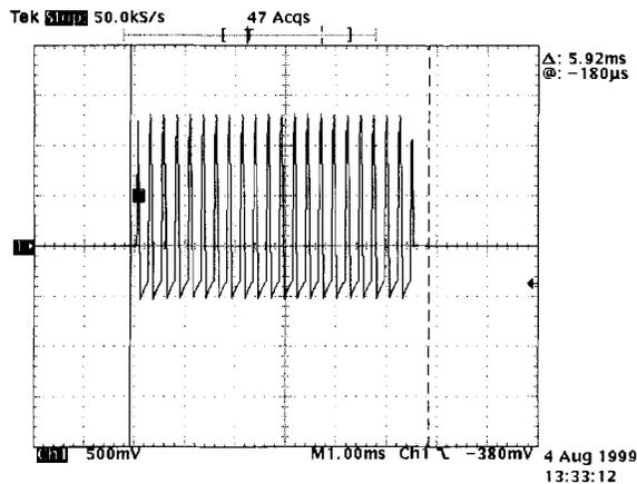
Fig. 2. Burst of Physio-Stim PEMF as measured within the field stimulation coils.
